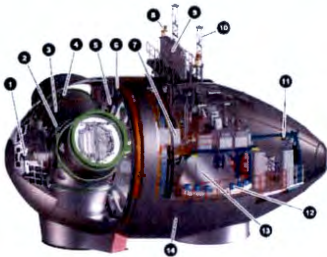
Fig. 2: View of E-126 EP4 nacelle
